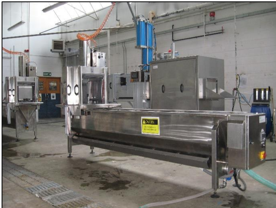
IMAGE 2: Two separate 'KiwiScour' scouring machines side by side with a single dryer behind.
